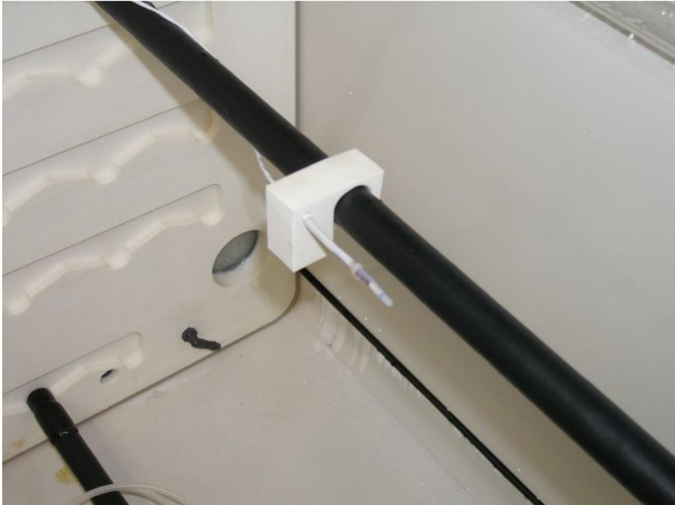
Unique: Temperature sensor positioned in the specimens zone allows highest accuracy and reproducibility of the climate conditions in the testing chambers
