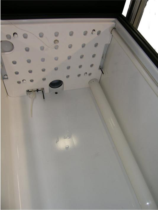
Air distribution pipes made from heat resistant PVDF for evenly drying of the specimens
