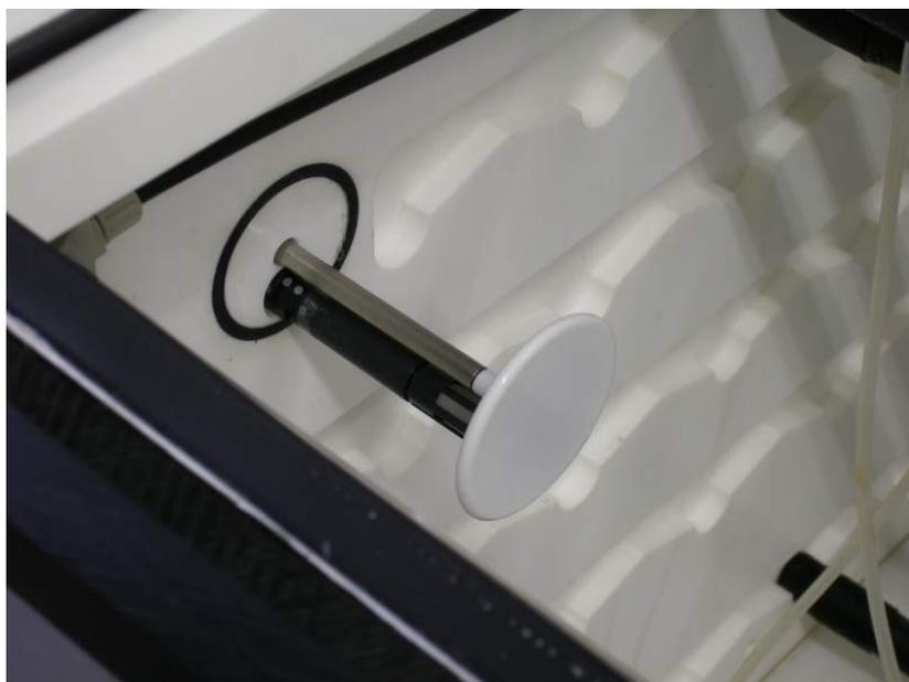
As the humidity sensor is not protected for instance by PTFE caps to achieve very short response on humidity changes. Due to the distribution by the spray nozzle there is a response of 2 seconds. The sensor will only be pushed pneumatically into the chamber if the humidity has to be controlled between 98% and  $< 20\%$  or if a low humidity set point has to be reached by forced air drying.
