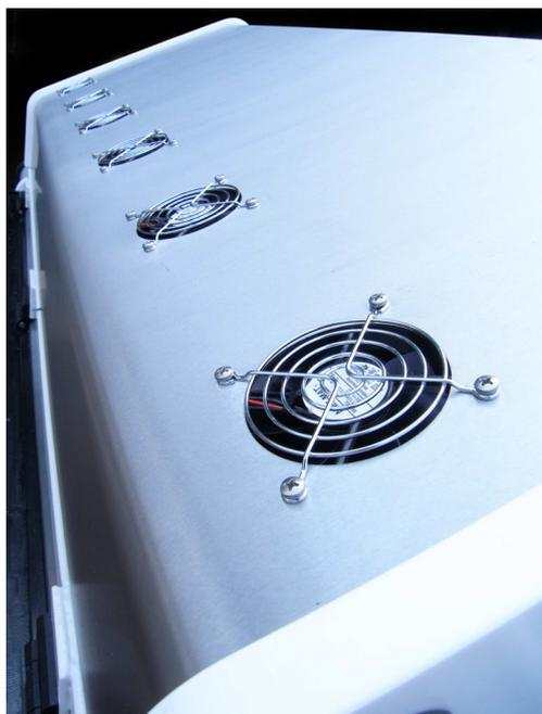
Fans in the back of the cover for cooling the roof thus the climate conditions inside the chamber allow a constant water condensation rate.
